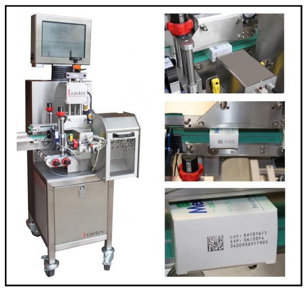
The Pharmacarton Coding Station is an established design for in-line, high resolution digital printing of lot, expiry, serialisation and 2D Datamatrix codes for pharmaceutical and medical cartons. The new design overcomes the problem of printing high density barcodes and 2D codes to ECC200/GS1 standards on line, by accurately controlling the carton during the print, vision & reject process.
