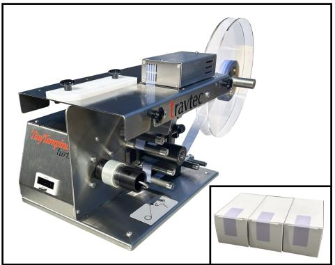
Tamper-evident labels semi-automatically applied to cartons
